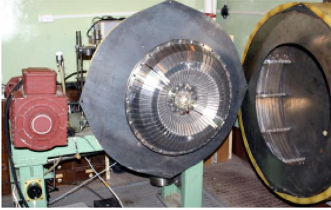
FIG. 1 (color online). Titanium channel and thermostatic cover.
