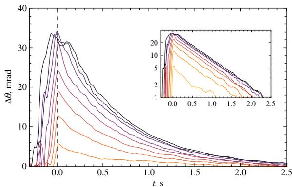
FIG. 4 (color online). Phase shift variations for the channel rotation rate  $\Omega = 10, 15, \dots, 40, 45$  rps (from bottom to top) in linear and lin-log (inset) scales.  $\nu = 97$  Hz.
