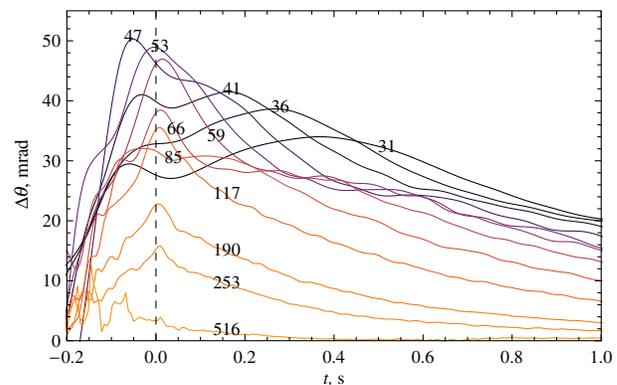
FIG. 5 (color online). Phase shift variations for the channel rotation rate  $\Omega = 40$  rps and different frequency  $\nu$ , shown near each curve.
