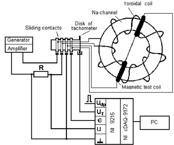
FIG. 2. Schematic circuit of the measuring system.  $U_{dp}$ ,  $U_T$ ,  $E$ , and  $U$  are the driving pulse, the tachometer signal, the electromotive force of the magnetic test coil, and the voltage, corresponding to the applied current.
