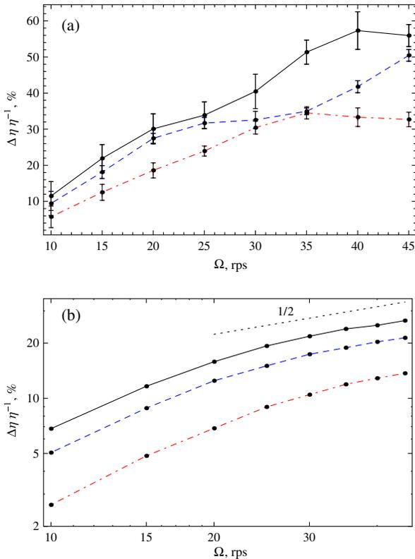
FIG. 6 (color online). Relative increase of magnetic diffusivity (percentage) versus the channel rotation rate  $\Omega$  at the end of braking (a) and at 0.7 s (b):  $\nu = 53$  Hz (solid, black line),  $\nu = 66$  Hz (dashed, blue line), and  $\nu = 97$  Hz (dash-dot, red line). Panel (b) is shown in logarithmic scale; dots show the power law “ $1/2$ .”
