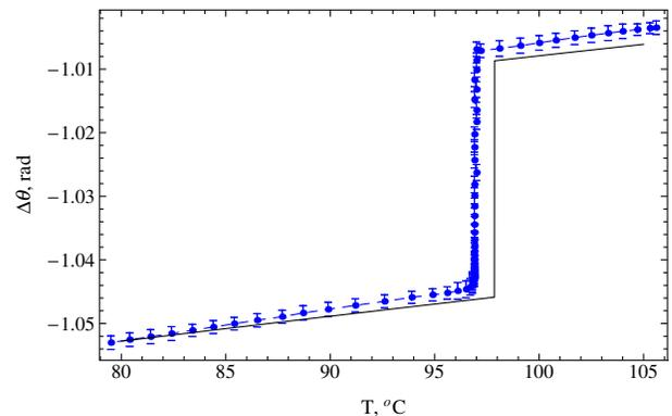
FIG. 3 (color online). Phase shift versus sodium temperature at frequency  $\nu = 97$  Hz: experiment (points) and simulations (solid line).
