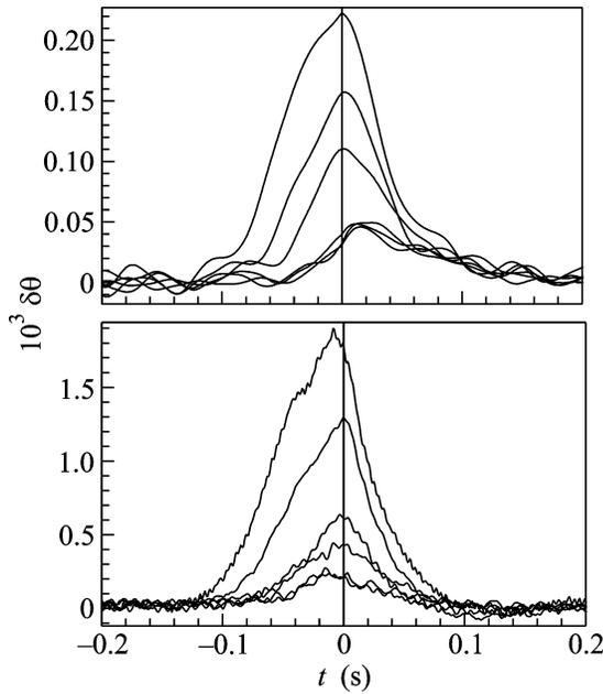
**Fig. 4.** Time dependence of the phase shift  $\delta\theta$  minus the deformation contribution for the initial torus rotation frequencies (from top to bottom) 55, 50, 45, 40, and 35  $\text{s}^{-1}$ . The resonant frequency is (upper panel) 166 and (lower panel) 964 Hz.
