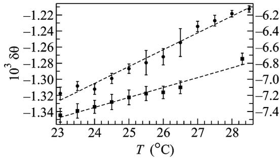
**Fig. 2.** Phase shift versus gallium temperature in the channel at a frequency of (upper data, left scale) 166 and (lower data, right scale) 964 Hz.
