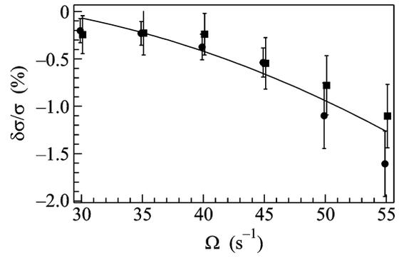
**Fig. 5.** Maximum relative deviation of the conductivity of the metal in the channel versus the initial channel rotation frequency  $\Omega$ . The resonant frequency is (squares) 166 and (circles) 964 Hz.
